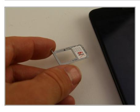
Remove the SIM card from the compartment using two fingers.
