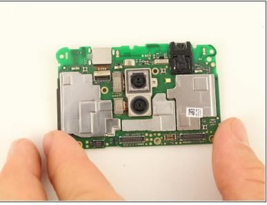
Remove the cable connecting the camera from the motherboard using a spudger or your finger.
