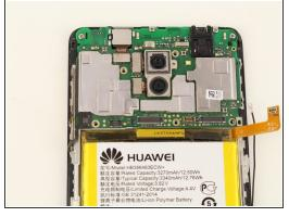
Pry the seven connectors off using a spudger or your finger.
