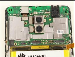
Remove the four 2 mm Phillips #00 screws.
