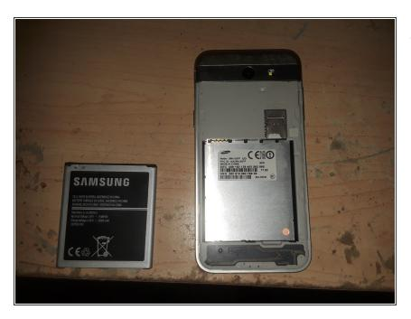
Pry the back off and take the battery out of the device
