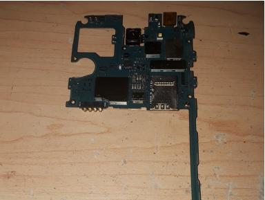
Gently go around the edge of the motherboard slowly prying it out, starting from the micro USB connector up.
