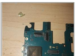
Lift the green tape (noted in red) that is over the camera connectors, and use the iFixit opening pick (or guitar pick) to lift up the tabs (noted in green) that hold the ribbon cable in place.
