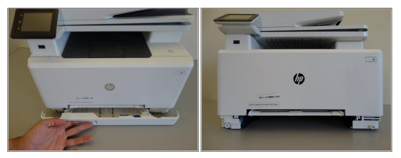
• Remove the bottom tray by pulling it until it fully is out of the printer.
