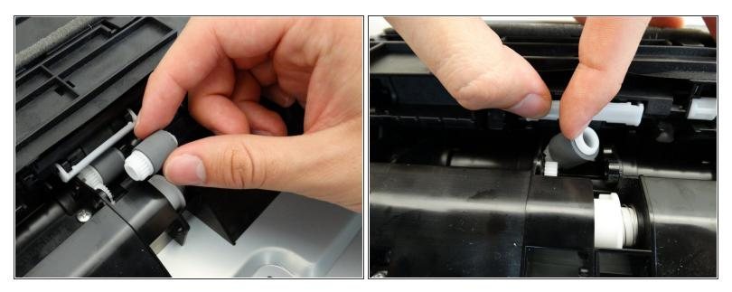
• Use your thumb to push in the white plastic hanging over the roller and use your index finger to pry the roller out.
