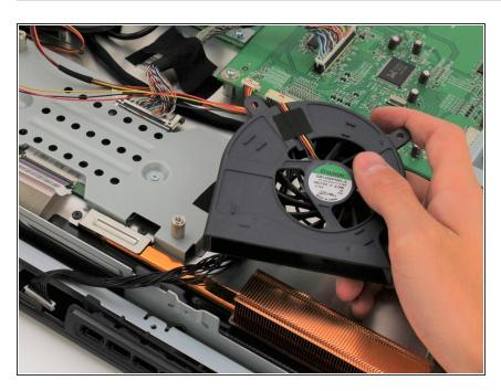
Remove the fan by lifting it up and off of the screw shafts.
