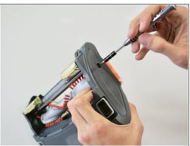
Turn the T10 Security Torx screwdriver counterclockwise to remove the 15mm screw.
