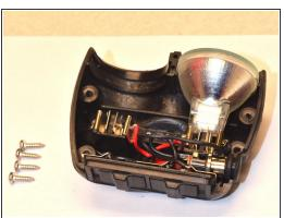
Obtain a <u>replacement bulb</u> and plug it into the empty socket.
