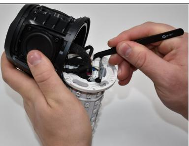
Use tweezers to pull the five connections off of the LED light display.
