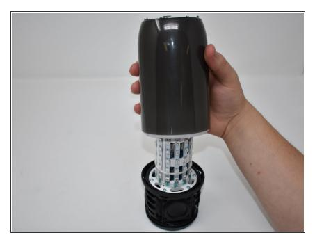
Pull the top section of the JBL Pulse 3 up. The outside casing to the JBL Pulse 3 should now be removed.
