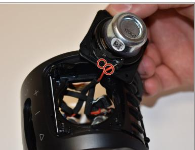
Pull out the speaker and cut the black and red wire with wire cutters. The speaker should now be removed from the JBL Pulse 3. To reassemble your device, follow these instructions in reverse order.
