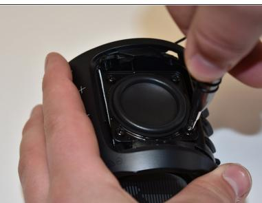
Using a Phillips #2 screwdriver, remove the four 10mm screws on the corner of the speaker on the side of the base of the JBL Pulse 3.
