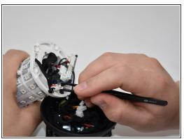
Pull out the motherboard slightly from the LED light display as shown. Using tweezers, unplug the three connections attached to the motherboard.
