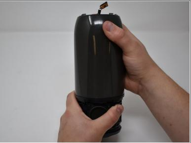
Peel off black, taped-on electrical lead from the inside side of the JBL Pulse 3.
