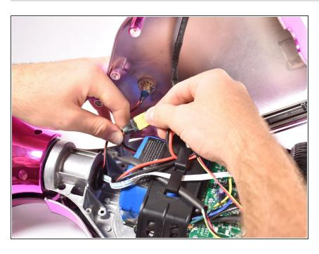
Lift the shell without the speaker grille and unplug the battery.
