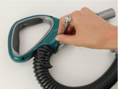
• Remove five 13.4 mm screws from the handle with a T20 Torx bit.
