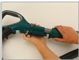
Press down on the handle release button and pull the wand away from the vacuum.
