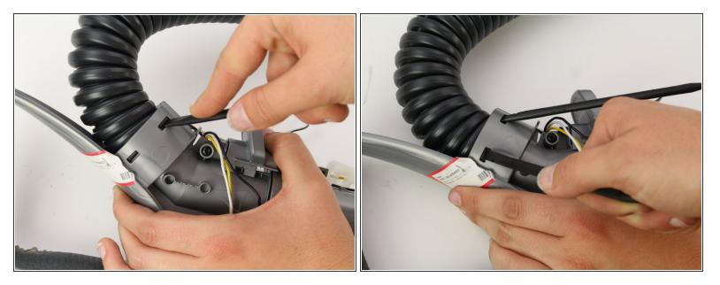
Using two spudgers, unclip the hose from the handle.
