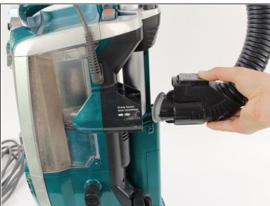
Press down on the hose release button and pull away from the vacuum
