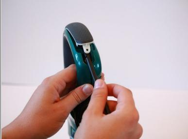
Remove the single 13.4 mm screw at the bottom of the handle grip and then lift the grip with a spudger.
