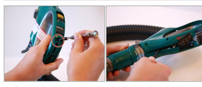
Remove the single 13.4 mm screw from underneath the handle grip. You are then able to open the handle using a spudger and pulling the pieces apart.
