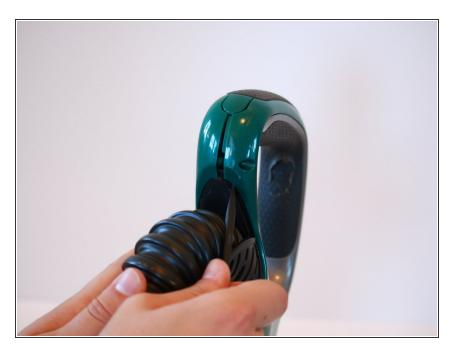
Run the spudger along the center seam of the handle, pulling it apart as you go.
