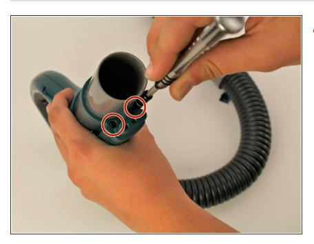
Using a T20 Torx bit, remove the two 13.4 mm screws from the front of the nozzle.
