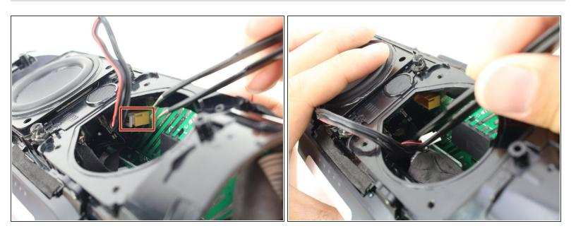
Grab the bundled cable connector that joins the speakers to the motherboard with tweezers.
