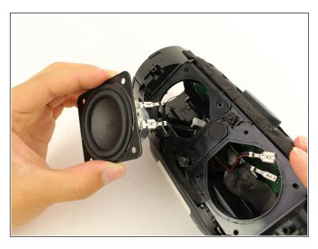
Now that the second speaker is disconnected from the motherboard, pull the speaker and wires out of the housing. To reassemble your device, follow these instructions in reverse order.
