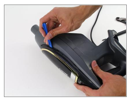
• Use the iFixit opening tool to remove the top component.
