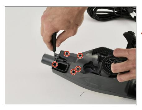
Remove the five 15 mm screws by twisting counterclockwise with a T10 Torx screwdriver.
