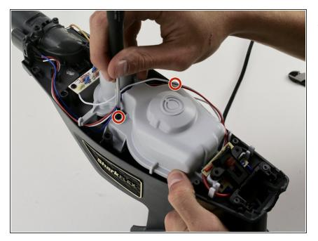
Remove the two 15 mm screws holding the motor cover by twisting counterclockwise with a T10 Torx screwdriver.
