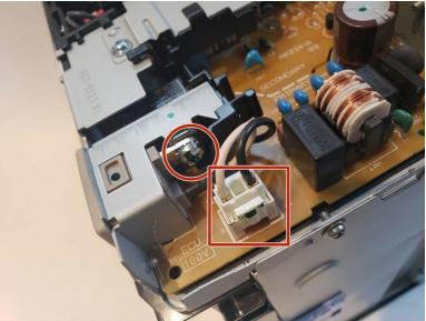
• The power plug will be held together with one Phillips screw 7mm and wire connection.
