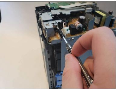
Unplug wire connector and unscrew the Phillips 7mm screw with #1 Phillips screw driver.
