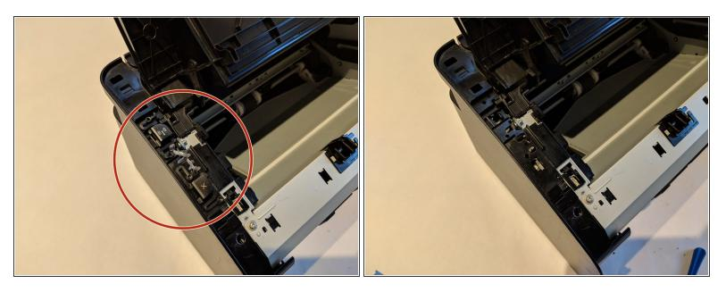
Once the housing is removed, remove the three buttons.
