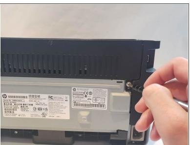
Unscrew the #1 Phillips screw 6mm on the back of the printer.
