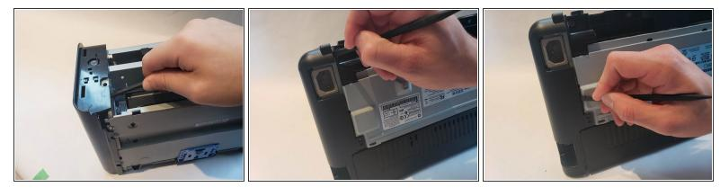
• Use the plastic spudger to remove the side panel. There are three main prying points as shown.
