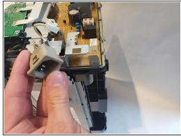
Apply pressure using spudger on top of the power plug to release it from metal housing. While doing that pull the power plug out.
