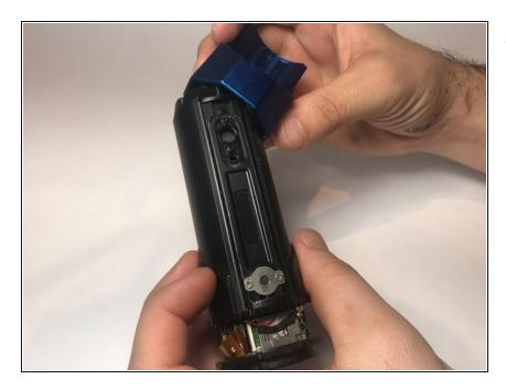
Finally, you can remove the body cover off and replace it with a new one if you have to.
