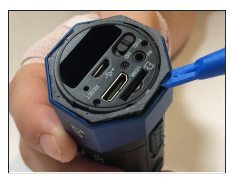
On the other side of the device, lift this black piece of cover that is underneath the cap, on the bottom side of the Ion Air Pro.
