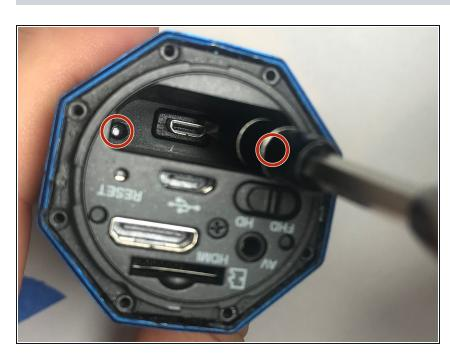
Remove two more screws, one on each side, inside this socket.
