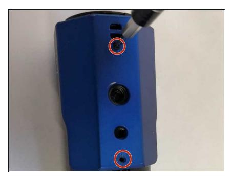
Next, unscrew the two screws located here.
