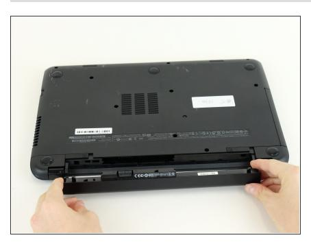
Pull on the battery to remove.
