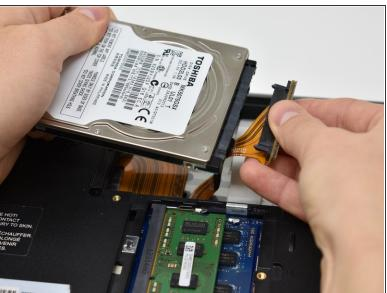
Gently lift the hard drive from the left side and disconnect the SATA connector from the right side.
