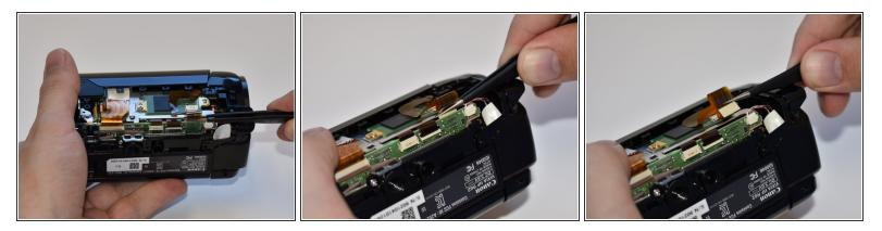
• Using tweezers, disconnect this ribbon cable by pulling straight out.
