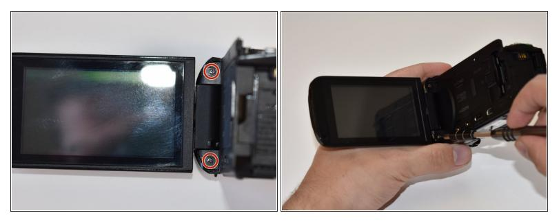
Remove the two 5mm Phillips #000 screws near the display panel.
