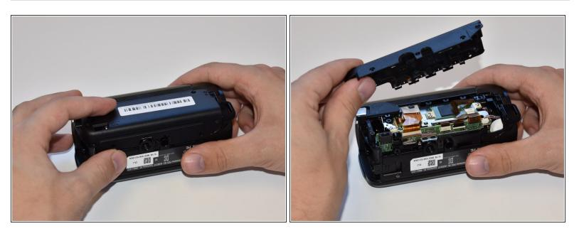
• Remove the panel opposite the display by pulling up perpendicular to the side.
