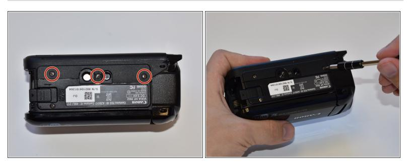
• Remove the three 5mm Phillips #000 screws on the bottom of the device.
