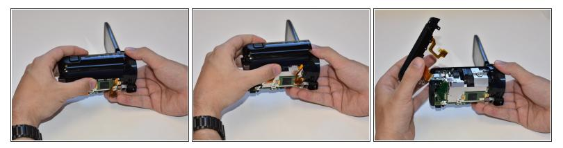
• Grasp the top of the camera and pull straight up to remove the top panel.
