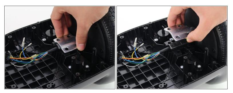
• Lift the metal retaining plate away from the motor shaft.
