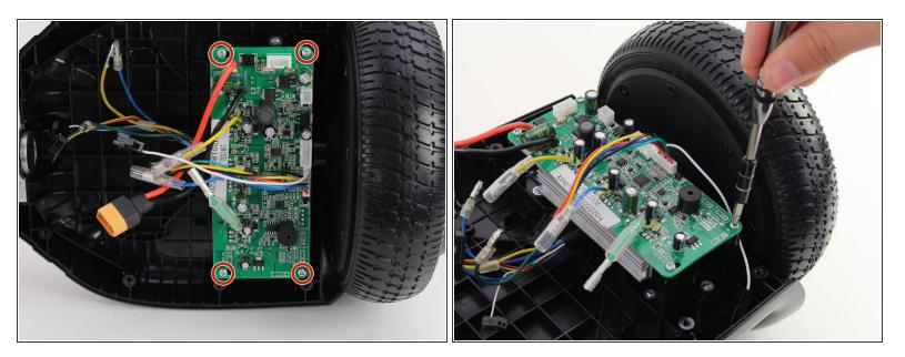
Remove the four 10mm screws with a Phillips #1 screwdriver.
