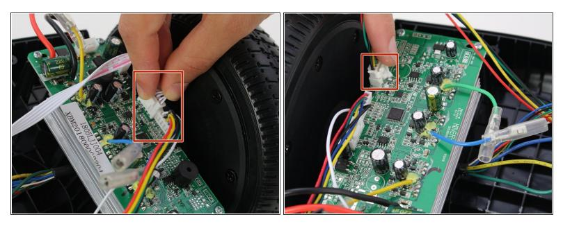
Remove the white cable from the sensor boards by disconnecting the cable on each side of the hoverboard.
