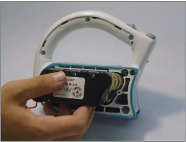
• Remove the battery by pulling it out of the slot it sits in.
