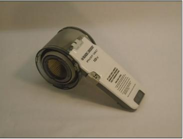
• To take off the nozzle, filter, and catch bowl first start off by pushing in the button identified with a red square and twist that part of the device toward the handle portion of the vacuum and it should click and pop off the chassis.
