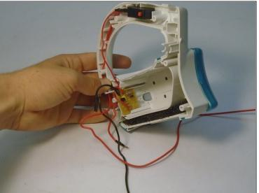
• Use a plastic opening tool to separate the two pieces of plastic.
