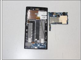
Use blue plastic opening tool to pry off the motherboard.
