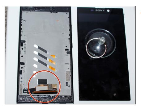
Unhook the screen sensor from the phone to detach the screen from the device.
