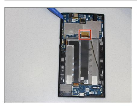
Unclip circuit connectors from phone to motherboard.
