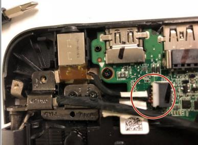
• Grab the wires and lightly pull to remove the power port from the motherboard.
