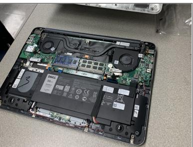
Pry out the back panel using the flat head side of the spudger.
