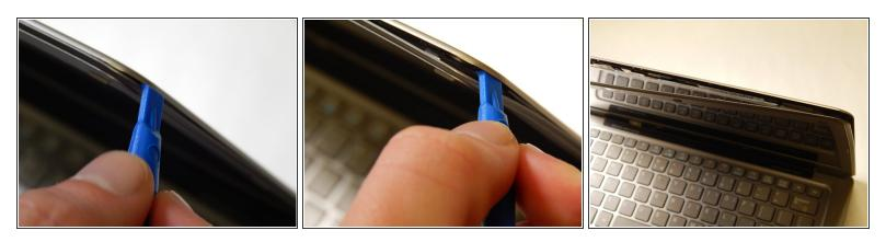
Use the plastic opening tool around the edges of the screen and remove the outer screen casing (the bezel).
