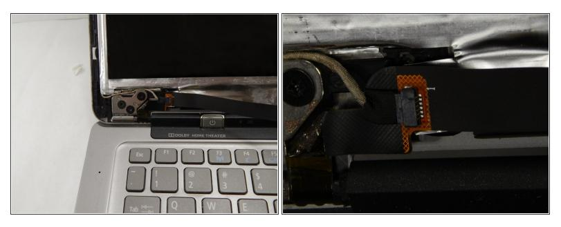
Disconnect the wire leading around the screen with a spudger or a plastic opening tool.
