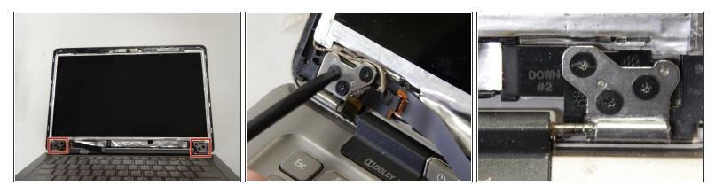
Locate the six 3 mm screws (there are three on each side of the screen). Remove them with the Phillips #0 screwdriver.
