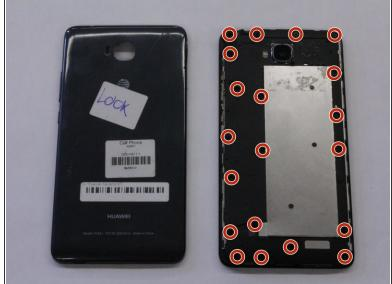
Use the Phillips head bit to remove 20 screws.
