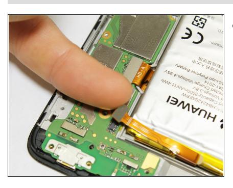
Carefully disconnect battery ribbon wire from lower left corner of circuit board.
