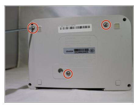
Remove the three 6mm Phillips #1 screws.
