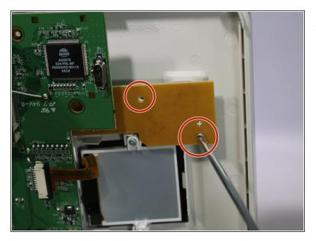
Remove two 8mm Phillips #00 screws from the yellow board.
