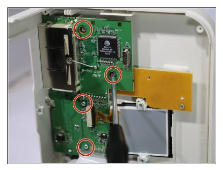
Remove the four 8mm Phillips #00 screws that hold the upper circuit board to the shell.
