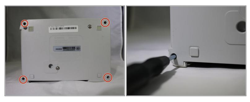
Remove the four 8mm Phillips #1 screws, located in each corner of the device.
