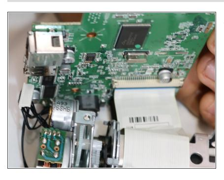
Lift the circuit board up off the lower assembly of the printer, exposing the wide, white data ribbon.
