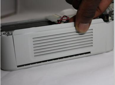
Lift the side panel off to expose the inside of the printer.
