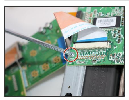
Remove the flanged Philips screw from the circuit board, located just under the large data ribbon connecting both boards.
