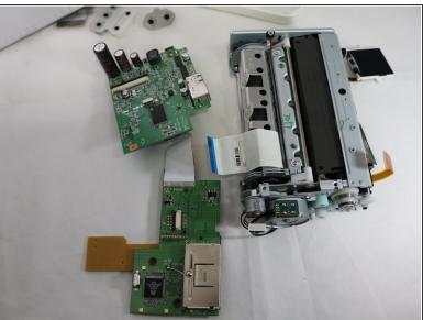
Pull the ribbon connector out of its socket parallel to the circuit board. All of the circuit boards should now be free of the device.
