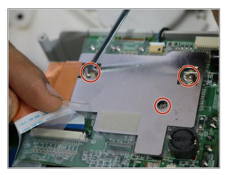
Turning to the lower half of the printer, remove the two 6mm Philips screws, and the 8mm Philips screw in the hole in the metal plate.
