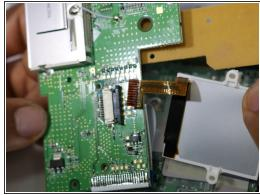
• To separate the screen from the circuit board, grasp the data ribbon cable near the base of the black connector on the circuit board and pull parallel to the surface of the board, toward the screen.
