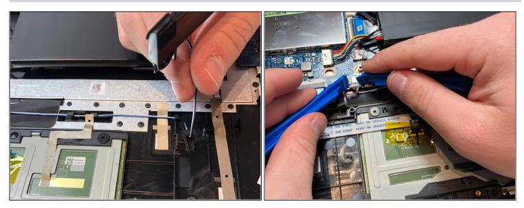
• Unwind the speaker wire from the plastic brackets. Once you have the wire completely unwinded, use two blue iFixit tools to disconnect the speaker chip from the motherboard.
