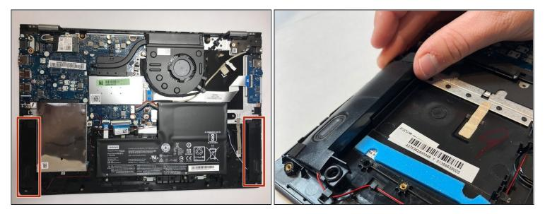
• Lift up on each speaker, one by one. The speaker should lift up with ease.
