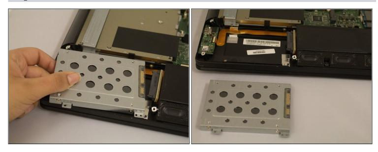
• Gently disconnect the Hard Drive from the connector cable. Lift it out and remove it.
