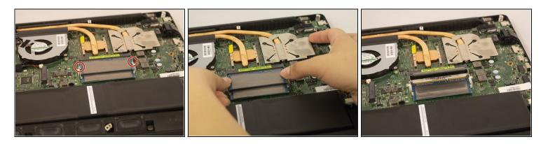
• Push both metal tabs away from each other on each side of the RAM farthest from battery so that the RAM will pop up.
