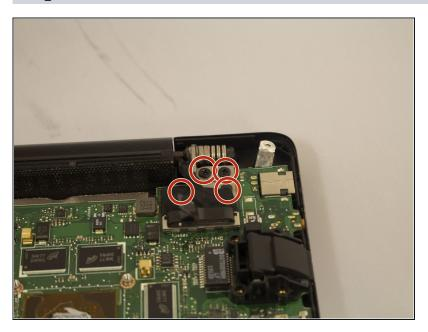
Use the Phillips #0 Screwdriver to remove the remaining four black 7 mm screws on the edge of the motherboard.
