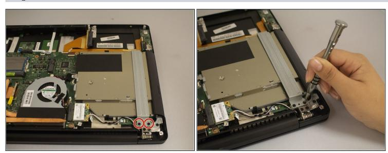
• Use the Phillips #0 screwdriver to remove the two 7mm Phillips head screws from the metal disc drive holder.
