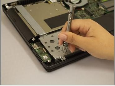
• Use the Phillips #0 Screwdriver to unscrew the four silver 5mm screws.
