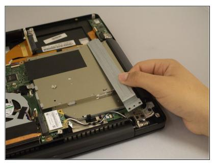
• Lift the metal disc drive holder off of the disc drive to remove it.
