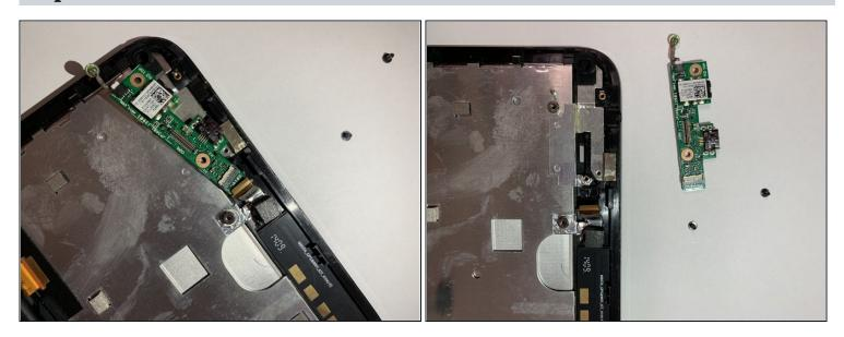
• Pull the DC board away while holding the ribbon cable.
