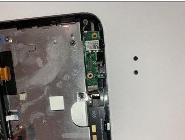
• Remove the two Phillips #000 screws holding the board down.
