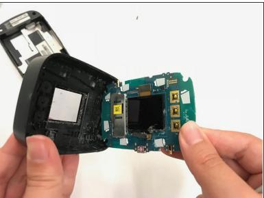
Using the metal spudger, gently pull out the motherboard from the plastic casing.
