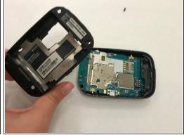
Using the metal spudger, pry the plastic casing around the device.
