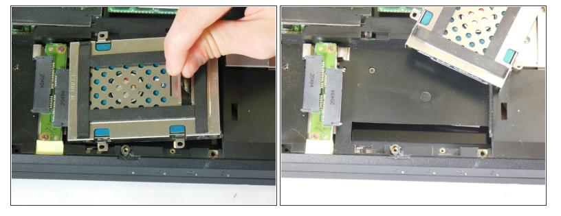
Remove the hard drive, lifting gently by the tab as shown.
