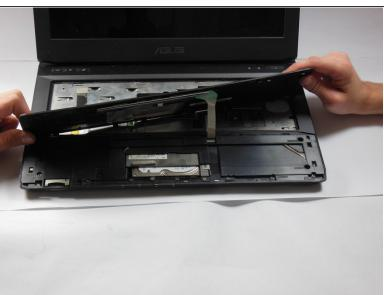
Use an iFixit Opening Tool to unclip the tabs on the sides of the laptop, just underneath the top plastic cover. Once one of them is off, it should pop off willingly. You may need to slide the tool around the edge like you did for the keyboard.
