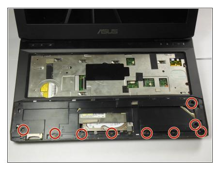
Unscrew the nine 2.5x7mm Phillips #0 screws highlighted in this image.
