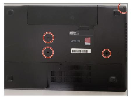
Unscrew the four 4mm screws using a Phillips #0 screwdriver.
