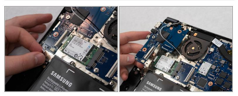
• Using your hands remove the cord that connects the speakers to the board you are removing.
