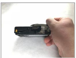
Move slider to opposite side which will allow battery door to open.
