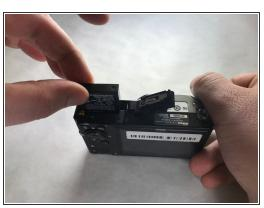
Compress the yellow clip away from the the battery until battery is released outward.
