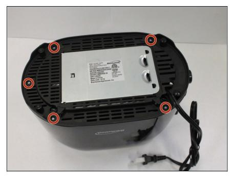
Remove the five 6mm screws on the bottom of the toaster with a Phillips #2 screw driver.
