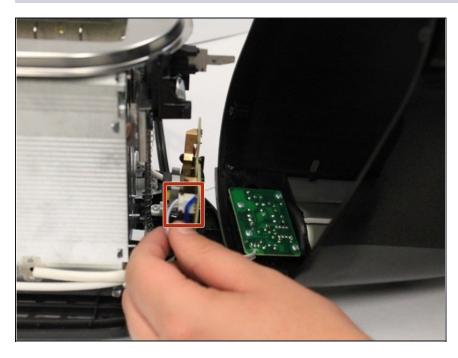
• Unplug the wire connecting the casing to the circuit board to fully remove the toaster casing.
