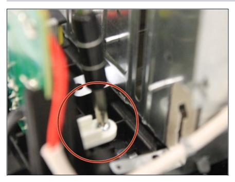
Unscrew the wire bracket with a Phillips #2 screw driver.
