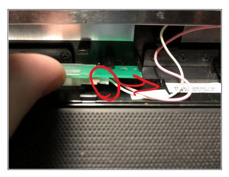
Disconnect the assembly from the chip located between the hinges by pulling the wires to the right.
