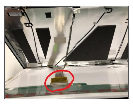
Disconnect the ribbon cable on the back of the display by peeling back the tape and then pulling down on the cable.
