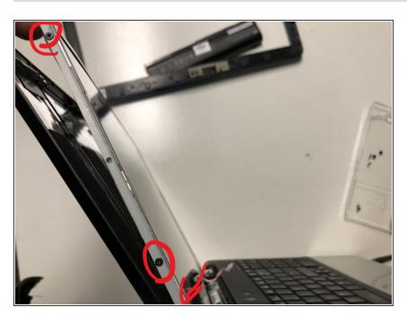
Pull the frame forward, and then unscrew the three screws on each side.
