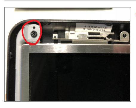
Unscrew the two screws in the top corners to separate the frame holding the assembly from the plastic of the lid.
