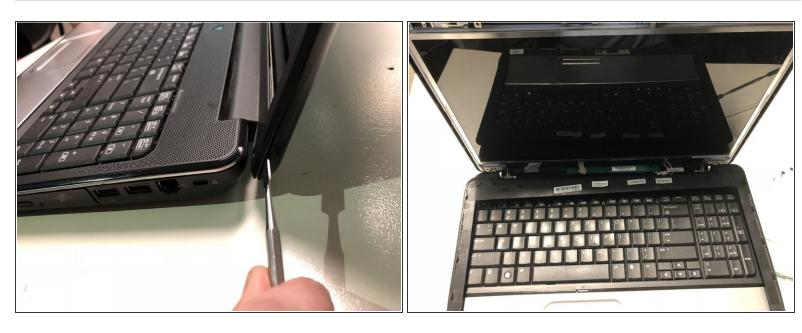
Use the metal spudger to gently pry the plastic faceplate off the rest of the display.
