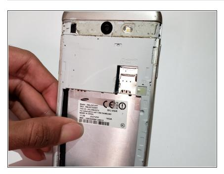
Turn the device over, and push firmly to separate the metal plate from the back paneling.
