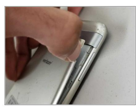
Insert your fingernail into the back cover removal slot and gently pull back until the cover pops off.
