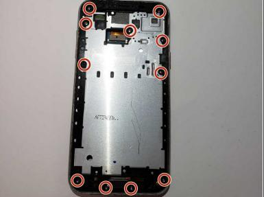
Using a Phillips #000 screwdriver, remove all eleven 5mm screws from the metal panel.
