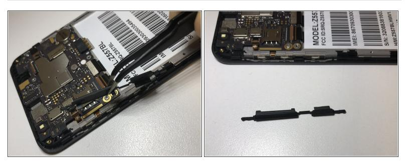
Carefully use a pair of bent nose tweezers to pull out the button cover. I should come out easily.
