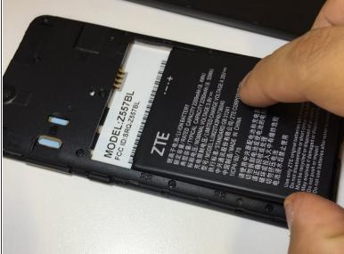
Remove the battery with an opening tool or fingernail.
