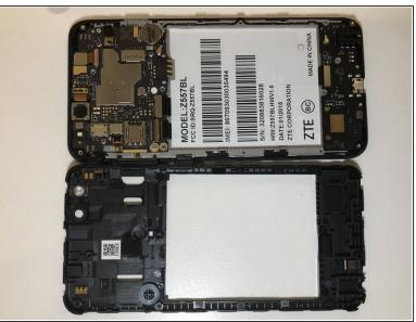
Unscrew all 16 screws from the mid-frame with a J000 screwdriver.
