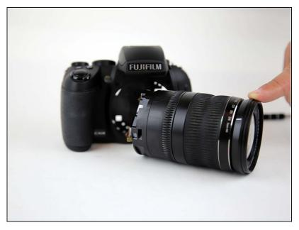
Un-attatch the current lens, and replace it with the new lens.
