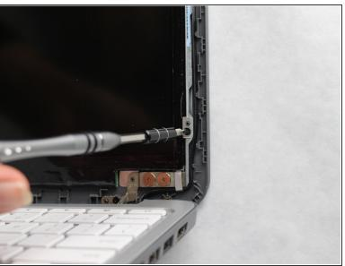
Remove the four black 3 mm screws along the left and right sides of the LCD screen using a Phillips #0 screwdriver.
