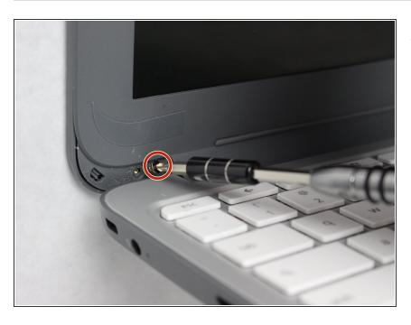
Remove the one 3 mm screw located underneath both adhesive layers using a Phillips #0 screwdriver.
