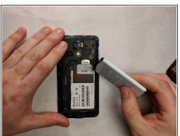
Remove battery using the spudger or your fingernails to pry the battery up out of the case.
