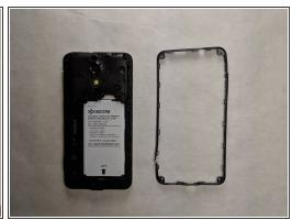
Remove the trim around the outside of the device by peeling it off with your hands.
