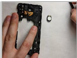
Remove the speaker from its location on the back frame using a spudger.
