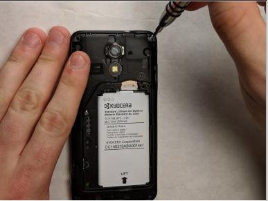
• Remove six Phillips screws (screw length of 5.35 mm and screw head diameter of 2.95mm) on the back of the device using a Phillips #000 screwdriver.
