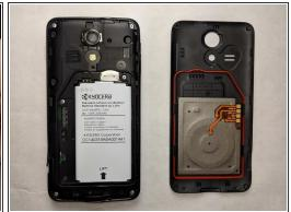
Remove the back plate of the device by popping it off with your fingernail or a spudger.
