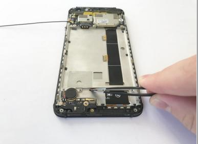
• Use a pair of tweezers to remove the orange data cable as shown.
