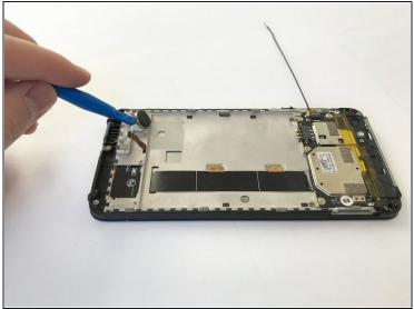
• To remove the vibrator, use the plastic opening tool to pry it out.
