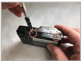
Remove the screws. There are two on each side, and four on the bottom. The black screws are 3.2 mm Phillips #000. The silver screws are also 3.2 mm Phillips #000.
