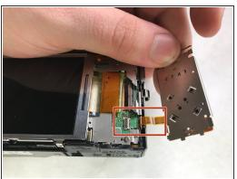
• Lift up on the black plastic tab(zero insertion force connector-ZIF) and gently pull the panel out to detach the ribbon cable from the camera body.
