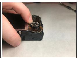
Press down and pull the Menu Wheel/OK Button panel towards the screen. This will release the panel from the slots.
