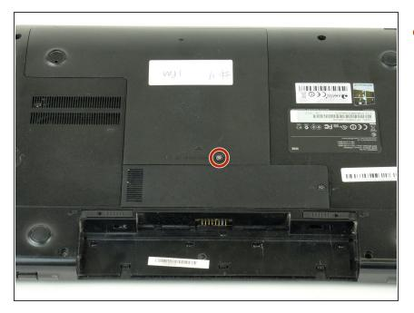
Remove the M2.5x5 mm screw with a Phillips #0 screwdriver.
