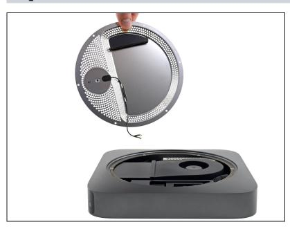
Remove the antenna plate from the Mac mini. Compare your new replacement part to the original part—you may need to transfer remaining components or remove adhesive backings from the new part before installing.
