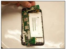
• Disconnect the connectors from the motherboard and gently remove the motherboard.
