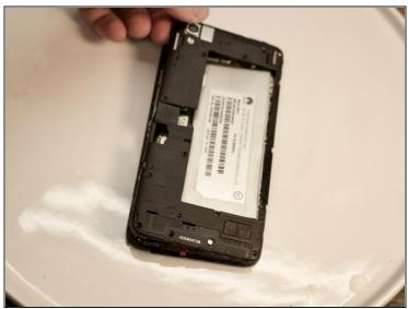
• Remove the 15 screws on the back of the phone with a Phillips #000 screwdriver.
