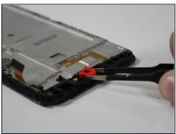
• Remove the microphone by lifting it out with the blunt <u>tweezers</u>.
