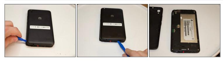
• Use the opening tool from the iFixit kit to get under the back cover and, gently separate the back from the front.
