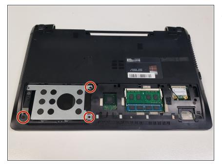
Use a Phillips #0 screwdriver to remove the 1.5 mm screws that hold down the hard drive.
