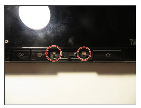
There will be two screws under the button you have removed. Use your Phillips #00 Screwdriver to remove these screws.
