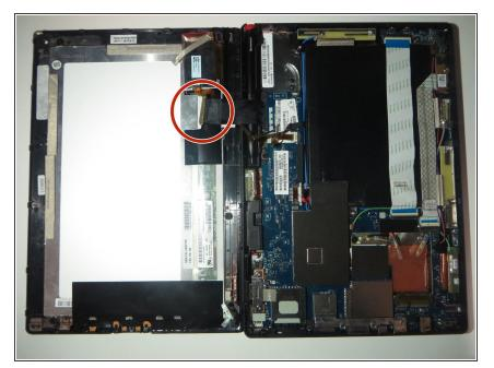
Before you separate the panels, there is a ribbon cable connecting the LCD to the motherboard. To avoid damage of the ribbon cable, lift the panel with the LCD from right to left like opening a book.
