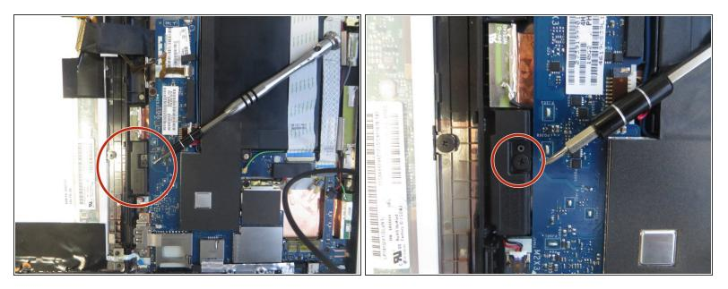
This is the speaker unit, and is being held by a screw. Use a Phillips #00 Screwdriver to remove the screw indicated by the red circle in the second image.
