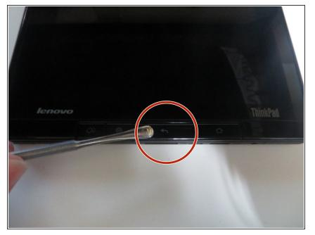
Remove the middle button by putting a plastic spudger or your fingernail underneath the button and lifting up.
