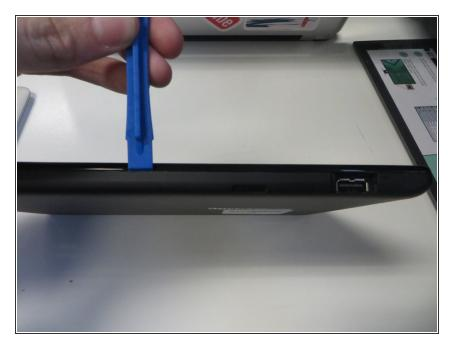
• With a plastic spudger or your fingernail, find the seam where the front and back panel connect and pry open from the bottom. After making a small opening, go around the device counter-clockwise.
