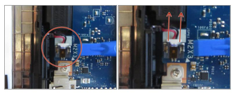
The speaker is still connected to the motherboard by a little connector. Using a plastic spudger or your fingernail, pry the connector to the direction marked by the two red arrows in the second image.
