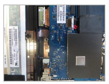
After removing the connector, you can now remove the speaker. Use your spudger or fingernail to lift the speaker up. The speaker should come out easily.
