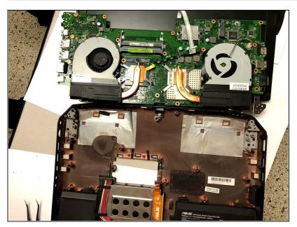
After lifting the motherboard up you can replace any component on it, such as the fans.
