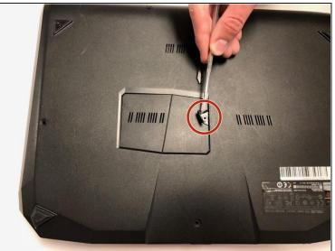
Lift the screw cover and remove the screw using a Phillips #0 screwdriver.
