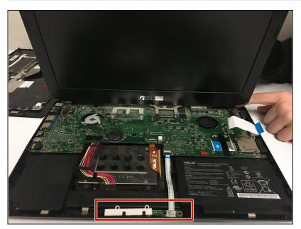
With the motherboard exposed, locate the Indicator Lights and their white plastic housing piece.
