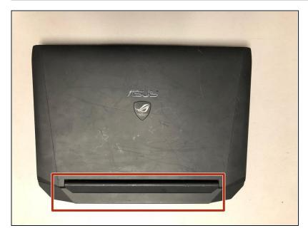
Gently pry the back hinge cover piece away from the device.
