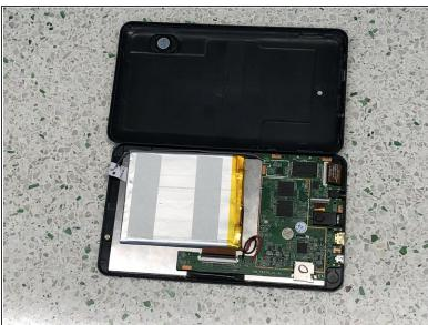
Open the device using a plastic opening tool.
