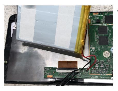
Disconnect the attached wires from the battery by desoldering the connections.
