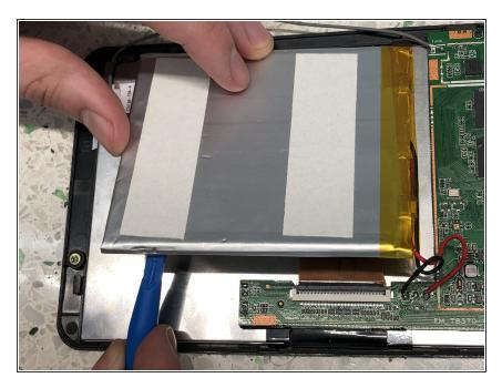
Lift the battery from the backing using a plastic opening tool.
