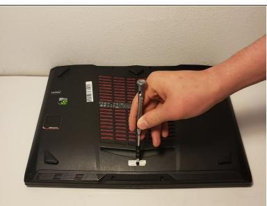
Remove the six screws on the back plate of the laptop using a JIS #0 screwdriver.
